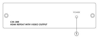
(1) Power LED: The LED indicator will illuminate when the unit is powered on.
