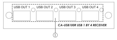
USB OUT 1~4: These slots are where you connect your devices, such as keyboards, mouse, printers, webcams or etc. with USB cables.
