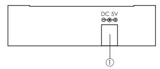
(1). DC 5V: This slot is where you plug the 5V DC power supply into the unit and connect the adaptor to an AC wall outlet.
