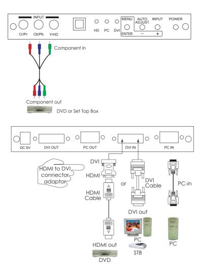
The CP-255D accepts component, PC and DVI inputs. The formats supported by these inputs are as follows:
