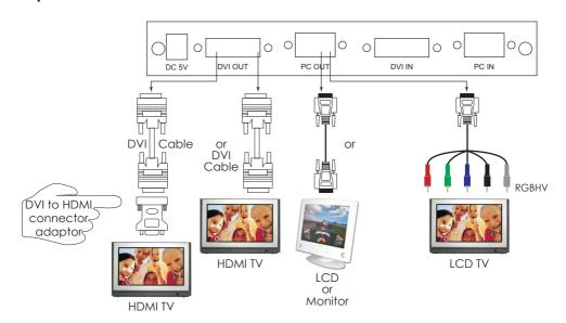
The CP-255D can output a variety of PC, SD and HD resolutions in both digital and analog format simultaneously.
