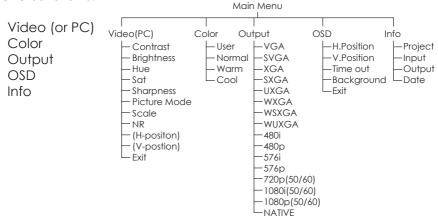
Use +, - button to move hightlight bar to your desired parameter, then press MENU/ENTER to enter into sub-menu of your selected parameter.
