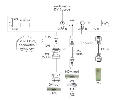
The CP-255H accepts component, PC and HDMI inputs with audio on each. The formats supported by these inputs are as follows:
