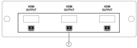
(1) HDMI Outputs 2/3/4: Connect each of the output ports to the HDMI display. When more than one output connected, the HDMI outputs play identical video signal simultaneously.
